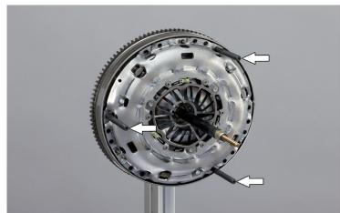
Fig. 2: Stud bolts for holding the spindle carrier
